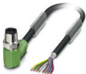
Sensor/actuator cable, 8-position, Variable cable type, shielded, Plug angled M12 SPEEDCON, A-coded, on free cable end, cable length: Free input (0.2 ... 40.0 m)
